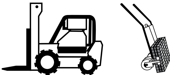
Figure 21. Fork lift and paver cart used to bring pavers to laying face.
